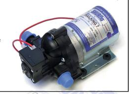
New improved 12v self-priming pump with built in pressure switch. Pump works automatically when water outlet is switched on and off. Aqua 8 will pump water vertically over 3m without priming. The pump is also resistant to limestone deposits and oxidation and is able to run dry without causing damage. New improved base plate with sound-absorbing feet that can be interchanged with previous pump models. 1 angle and 1 straight hose connector supplied for 13mm diameter flexible hose.
