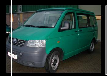
Superflat elevating roof by Reimo. We use this elevating roof on the T5 as it's the best on the market. The optional roof bed system gives ample space for two adults. With removable panels with flyscreens fitted into the side panels of the canvas this is the best place to sleep on a warm summers night to enjoy the view
