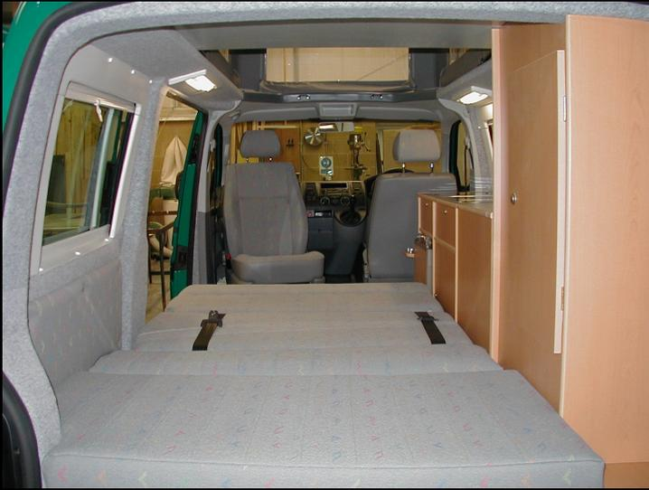
The Seat / Bed system slides on tracks fitted to the floor which makes the change from seats to bed as easy as possible in a vehicle of this size with no cushions to shuffle around.
